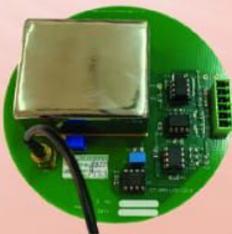
Pico Ampere Signal Conditioning Board 4pA - 1 \mu A | 4 - 20mA
