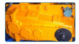
The gear box casings are fabricated and stress relieved. All the pinions & gears are supported on Ball / Roller bearings. The pinion & gears are suitably hardened to take care of wear.
