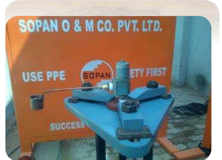
Safety Relief Valve Testing
