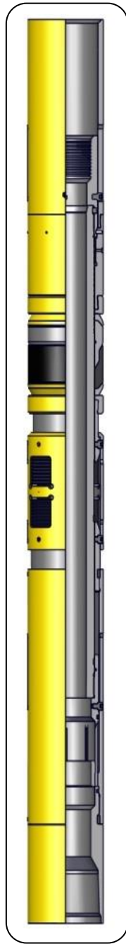
Model "BRSB" Retrieval Hydraulic Seal Bore Packer Product No.: BI 646-88
