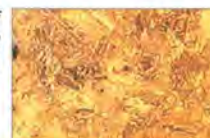
Microstructure of Martensitic Stainless Steel ASTM A 743 Gr. CA6NM.
