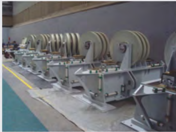
Foundation Beams manufactured as per design of Rexroth-Bosch, Netherland for Goa Shipyard.
