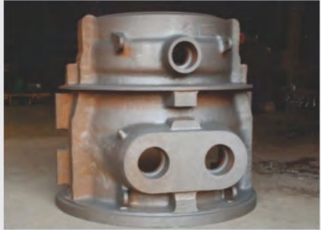
Inner Casing - Steam Turbine
