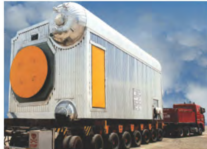
77 TPH Package Boiler being dispatched for installation at Longview, Madsville, West Virginia, USA.
