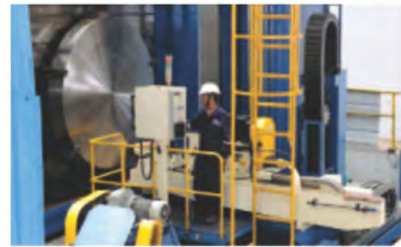
Gun Drill for drilling tube sheets up to a thickness of 1000 mm.
