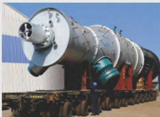
<<< Secondary Reformer supplied to Technimont, India for NFL Nangal, India.
