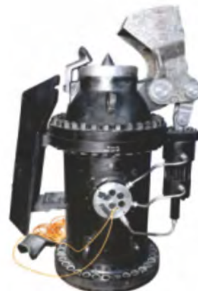
Nozzle Deflector Assembly manufactured as per design of Voith, Germany.
