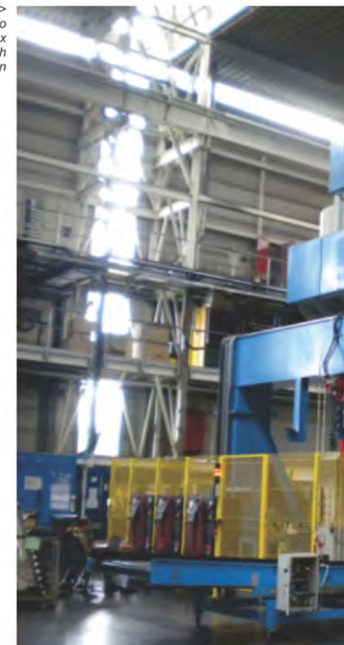
>>> 2000 Tonne Transfer Press supplied to Brandl, Germany with Bed Size of 6100 mm x 2800 mm & 5 station Robotics Transfer with 64 Tonne capacity die-cushion at each Station
