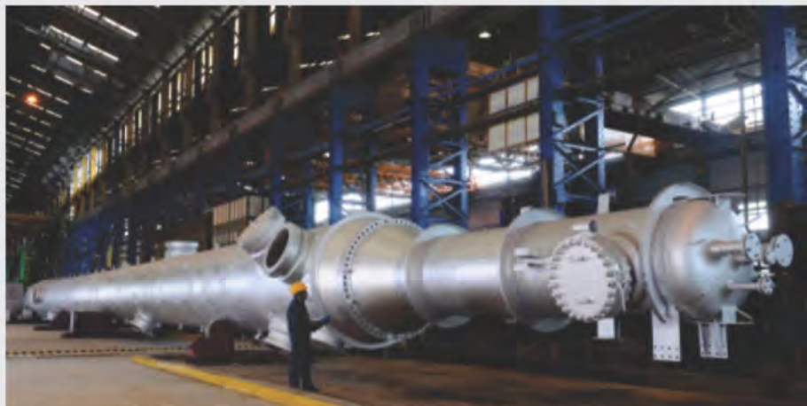
CCR Reactor (1 1/4 Cr - 1/2 Mo) supplied to BPCL Kochi Refinery. Similar Reactors have been supplied to HPCL, Mahul Refinery and BORL, Bina Refinery.
