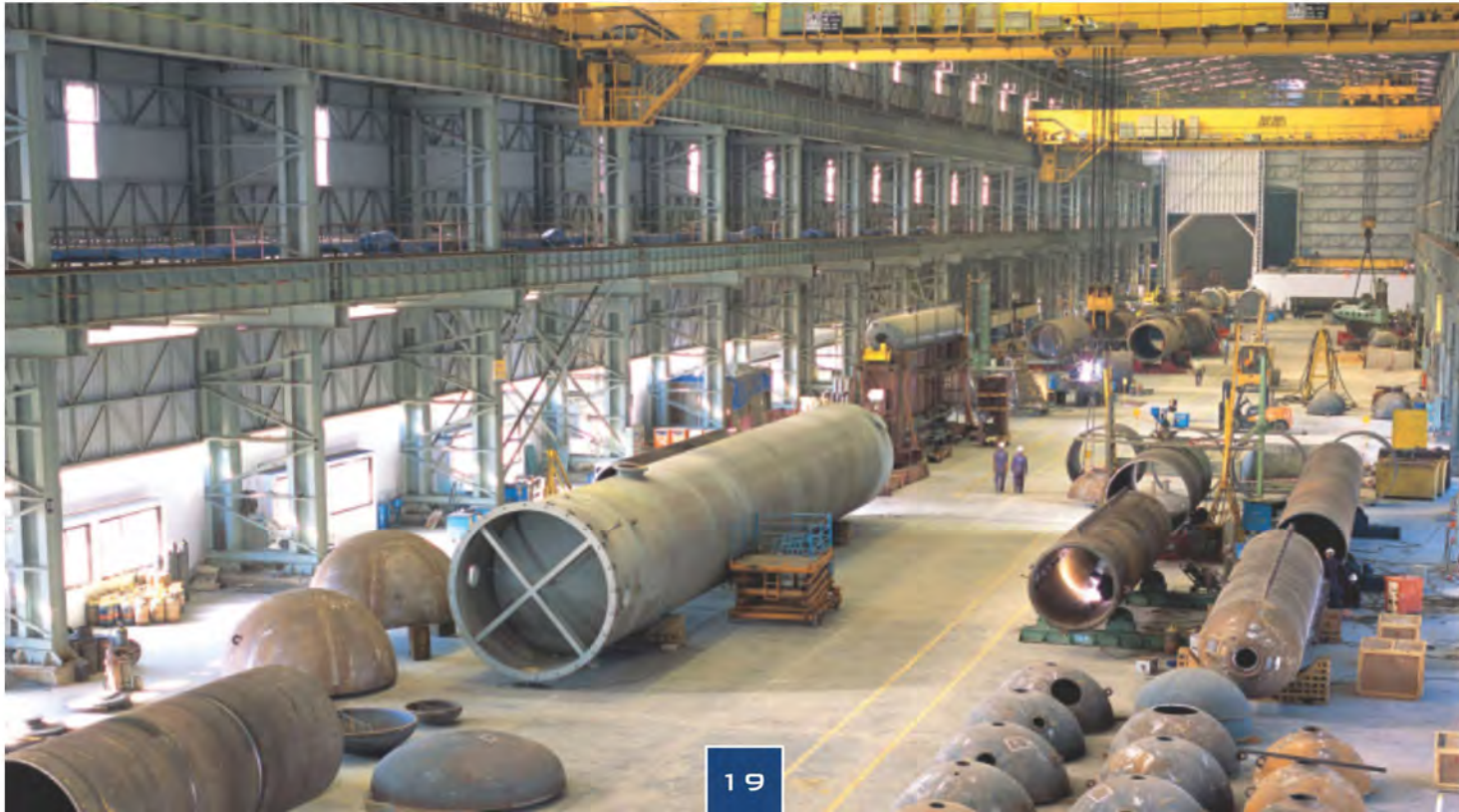
Heavy Shop at Dahej with a crane lifting capacity of 300 Tonnes and under hook height of 14 M.
