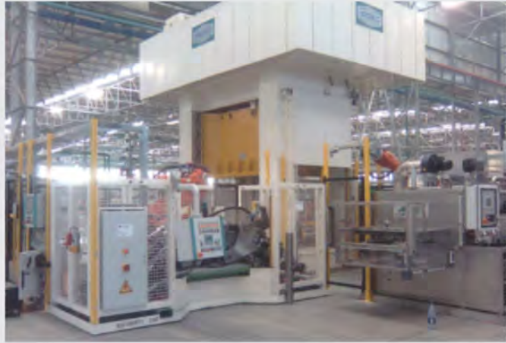
<<< 630 Tonne Hydraulic Press supplied to Benteler, South Africa comprising customised Hydraulic Press interfaced with Robotic Automation.
