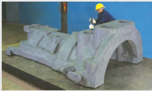
Outer Casing - Steam Turbine
