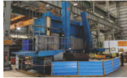
VTL for machining up to 6300 mm OD and 3500 mm height.
