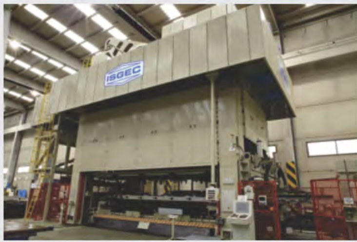
<<< 2500 Tonne Transfer Press supplied to CIE Automotive, Spain with Bed Size of 7000 mm x 2800 mm & equipped with 3-axes Electronic Transfer System complete with Feed Line.
