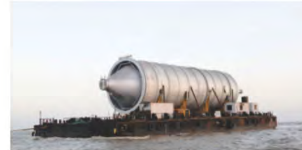
Coke Drums supplied to MRPL for their DCU facility through Punj Lloyd. 4 Nos. of such SS Clad Coke Drums were supplied having a diameter of 9144 mm, length of 41,600 mm and weighing 454 MT each.
