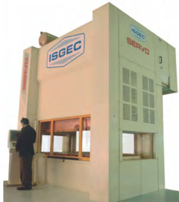
>>> 2000 Tonne Transfer Press supplied to Brandl, Germany with Bed Size of 6100 mm x 2800 mm & 5 station Robotics Transfer with 64 Tonne capacity die-cushion at each Station
