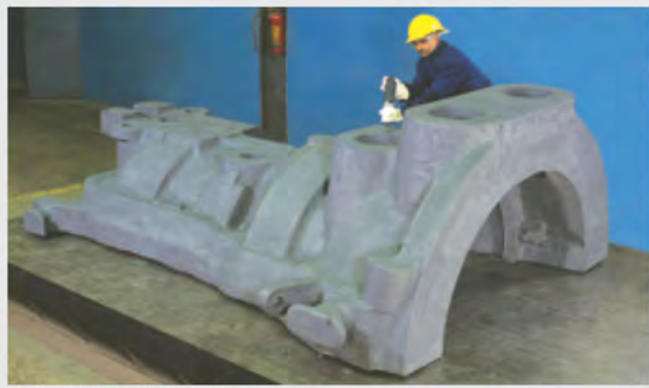
Outer Casing - Steam Turbine
