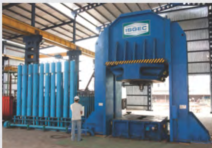
<<< 12500 Tonne Hydraulic Press with large Accumulator Bank is being used for Hot & Cold Forming of High Tensile Steel Plates for Defence & Aerospace Applications.
