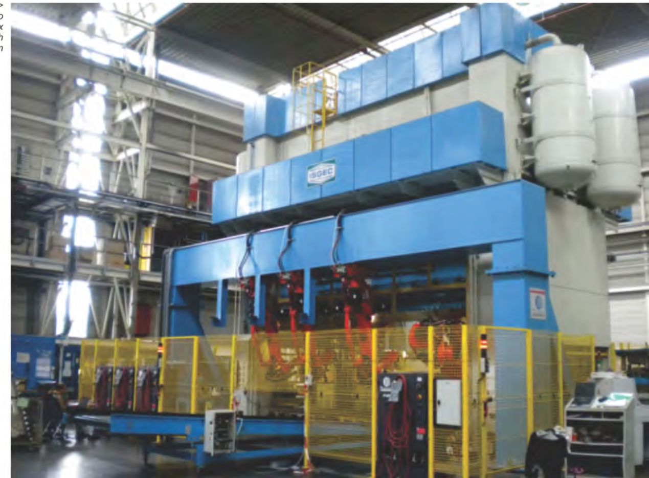
>>> 2000 Tonne Transfer Press supplied to Brandl, Germany with Bed Size of 6100 mm x 2800 mm & 5 station Robotics Transfer with 64 Tonne capacity die-cushion at each Station
