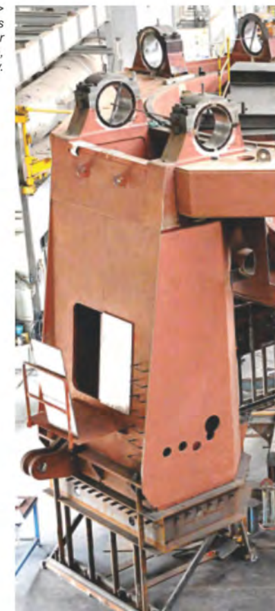
>>> Mill Stands manufactured as per design of Loesche, Germany.
