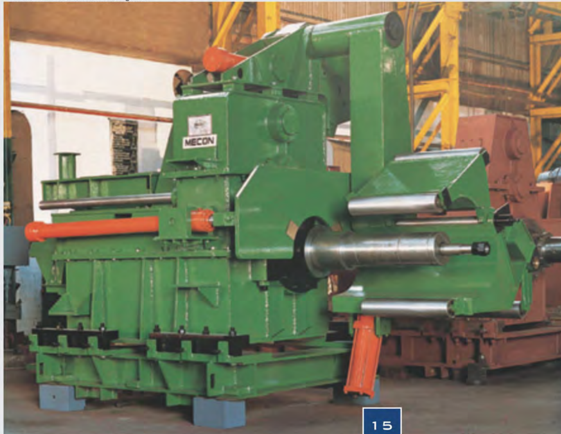
Tension Reel for a Cold Rolling Mill.
