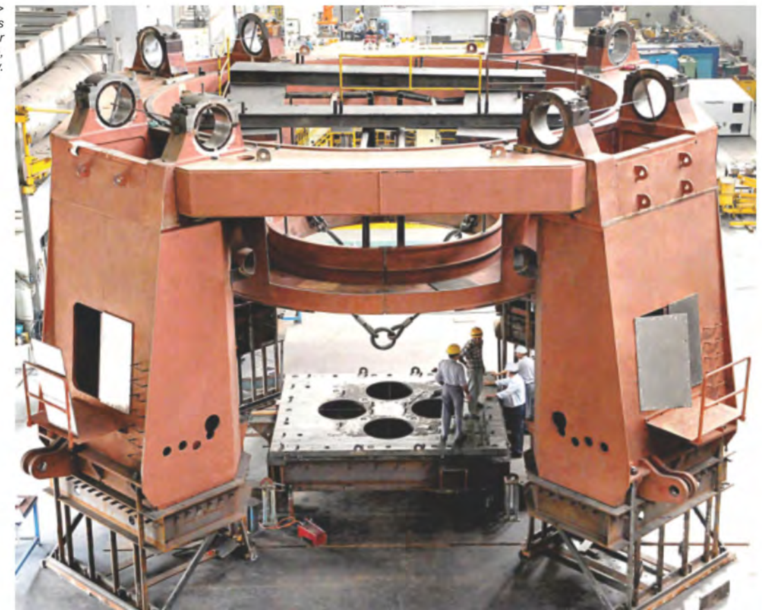
>>> Mill Stands manufactured as per design of Loesche, Germany.
