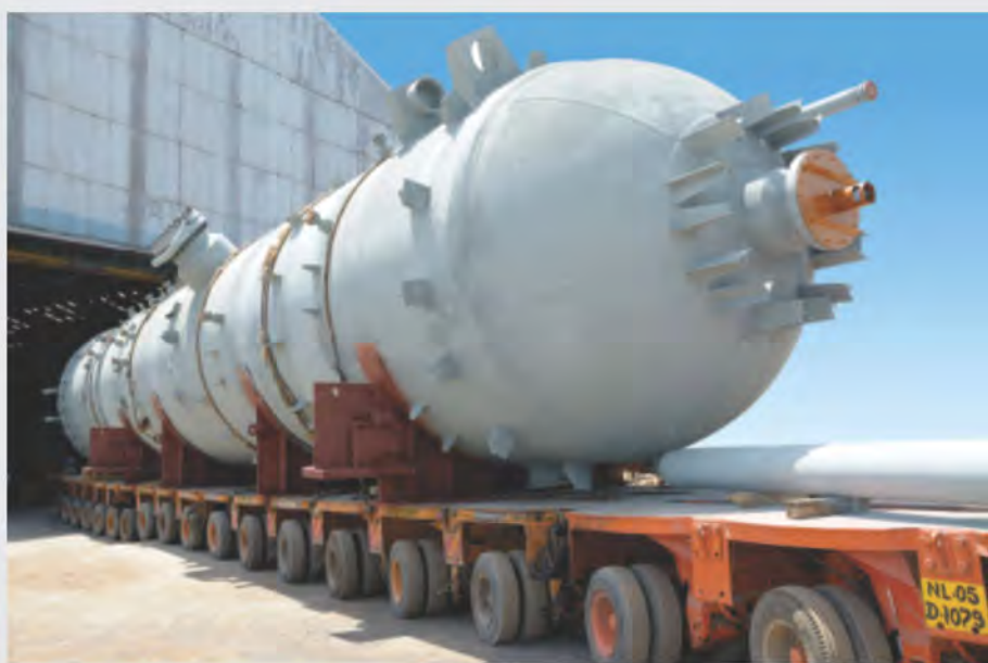
2 1/4 Cr-1 Mo Hot Separator for HMEL, Bhatinda Refinery, India.
