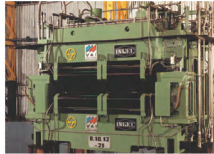
The Strand Guide Segment shown in this picture is a part of a Continuous Caster Plant. We have supplied Mechanical Equipment for CCP to the design of SMS-Demag, Germany and Voest Alpine, Austria.
