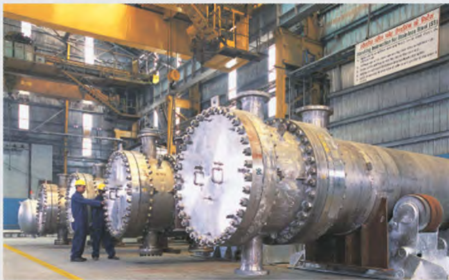
SS Exchangers supplied to Lurgi, Germany for Hydrogen Generation unit at the Netherlands.
