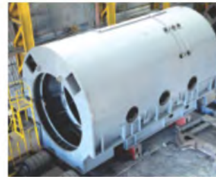
Stator Frame for 250 MW Power Plant for BHEL, Haridwar, India.
