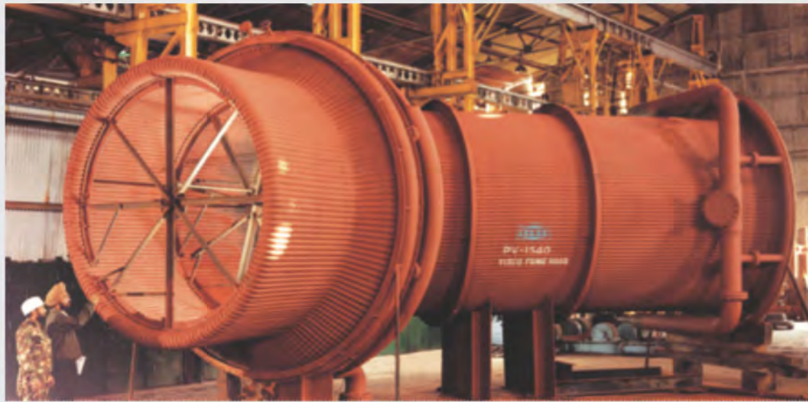
This Fume Hood is a part of the Gas Cleaning Plant for a Blast Furnace. We have supplied Fume Hoods to the designs of Clecim, France and Davy Ashmore, UK and these are installed in all major steel plants in India. We have manufactured both tubular and plate type Fume Hoods.
