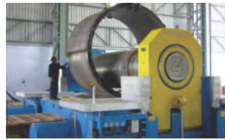
Haeusler Bend Roll with a Cold Rolling capacity of 250 mm thickness.
