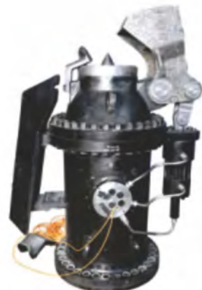
Nozzle Deflector Assembly manufactured as per design of Voith, Germany.
