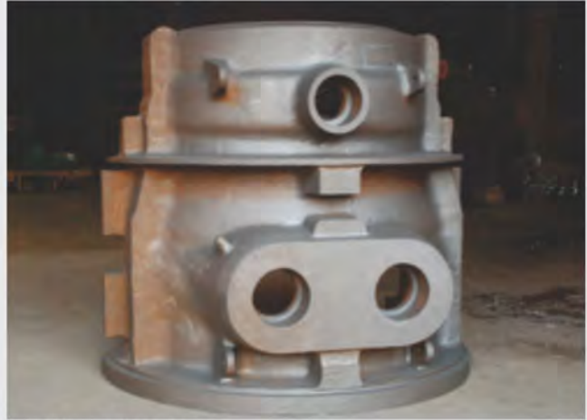
Inner Casing - Steam Turbine
