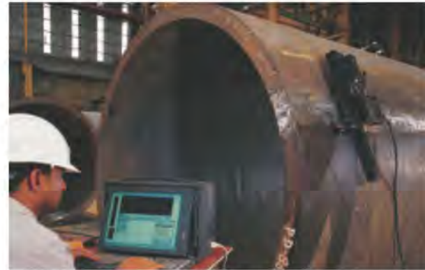
Mechanised Ultrasonic Testing of a 100 mm (4") thick drum.
