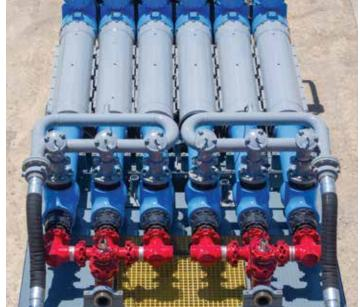
**More Horsepower, Same Footprint** – With twice the horsepower of a conventional pump unit, the 6,000 HP *DuraStim* pump occupies the same 3-axle trailer footprint. As a result, the pump:
