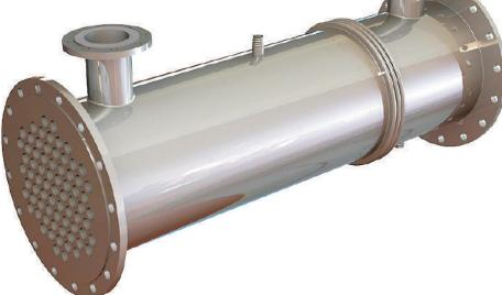
Shell Tube Heat Exchangers have a wide range of applications oil refineries, as well as other chemical processes. They aid in high-pressure applications. They are made up of a large pressure vessel called the shell which has many tubes inside it. This is the reason it is known as "shell tube heat exchanger". The set of tubes is called a tube bundle comprising various types of tubes like plain, longitudinally finned, et al.
