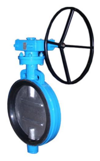
Wafer type butterfly valve with an integrally bonded elastomer liner. Requiring absolutely no form of maintenance the **UNIMAC** is a perfect "Fit and forget" valve. Available with either a flangeless or lugged body, in a size range of 50-600 mm,a pressure rating of up to PN 16 and offered with latching lever or actuation as well as different combination of disc and seat materials, "UNIMAC" is a truly versatile valve.
