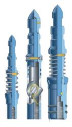
**Latches** are available in a wide range of designs for use with retrievable gas lift and circulation valves to be installed in side pocket mandrels and make it easy to install and remove Gas Lift Valves, very little force is required to operate these latches to keep the wireline time to a minimum. These are available in 1"-1.1/2" sizes.
