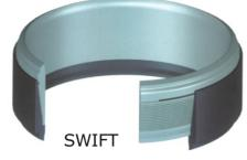
The Swift is a heavy-duty threaded connector for use on exploration and platform casing strings where high strength and pressure integrity are important. Compared to other connectors of similar performance, the Swift requires very low make-up torque and can be assembled using standard rig tongs. It has strength characteristics higher than those of the casing Pipe.
