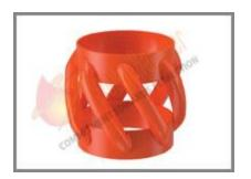
SledgeHammer's Spiralizor is designed specially for highly deviated or horizontal wells. Ideal for use with Liner Hangers. The steel construction ensures extra strength and superior toughness. The boat shaped Spiral fins minimize Drag Forces while running pipe. The fins glide smoothly in the low side of horizontal bore holes.
