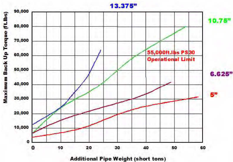
Figure 2.1: Maximum torque PS30 = 55,000 Ft. Lbs (74,570 Nm)
