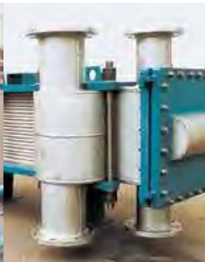
Zinc liquor heater
