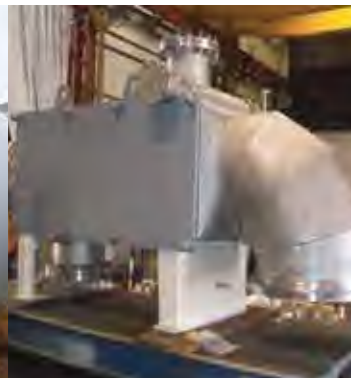
Condenser on methionine reactor
