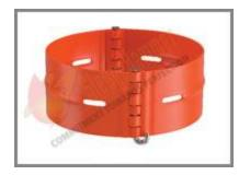
The Hinged Spiral Nail Stop Collar comprises of two parts and hinged at two ends making an angle of 180 degree. This hinged Stop Collar has an internal groove and these are available in 4 1/2 " to 20 " sizes+ any sizes in which a spiral locking pin is inserted. This tightens the collar to the casing firmly.
