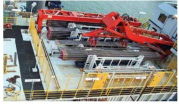
Automated pipe racking system on cantilever deck with gantry crane and pipe boxes (man free no-go area)
