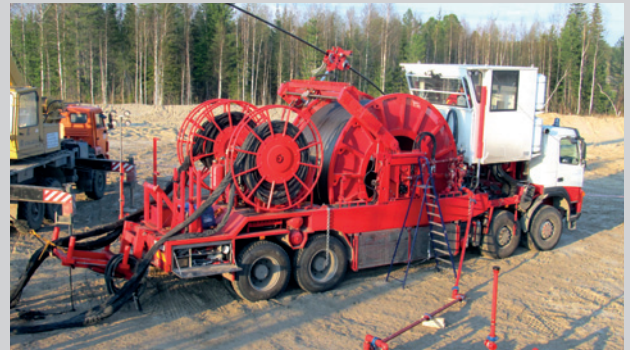
Truck Mounted CTU built for Arctic Conditions
