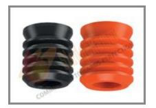
Sledge Hammer Cementing plugs are manufactured of graded rubber that is fused upon a composite or Aluminum core. This top plug can be used when dual plug system is not required and Bottom cementing plug can be used when dual plug system is required. These plugs are completely PDC drillable. Operating range of temperature with Aluminum core is up to 200 degree Fahrenheit.
