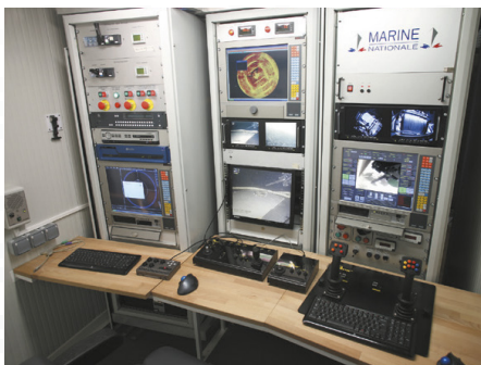
The 20 ft H1000 control unit and service container allow to control the ROV/LARS/TMS from the surface, and visualize in real time data brought by vehicle's sensors.
