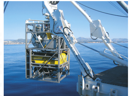
The Tether Management System (TMS) stores the tether cable and deploys the ROV at working depth for a larger operational radius.
