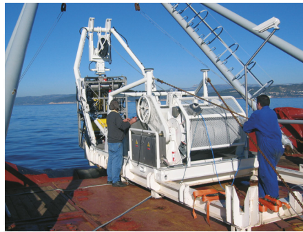
The LARS main function is to launch and to recover both ROV and TMS aboard the ship thanks to an A-frame allowing 3,50m overboard deployment.
